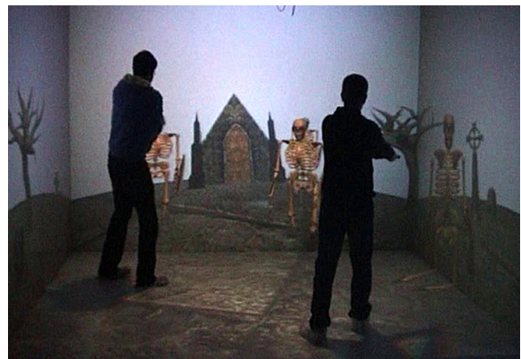
Figure 1: Two students play a collaborative game on a CAVE. The video game (both art and logic) was quickly created using the visual editing tools of Blender. Then, our easy-to-integrate BlenderCAVE framework manages a distributed rendering architecture based on the Blender Game Engine that generates the video output for all screens in the CAVE.
